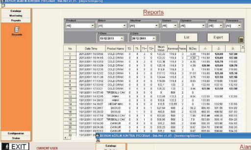
Weighing records in any entered two dates are filtered by various user's defined criteria such as product, batch, machine, operator, etc.
